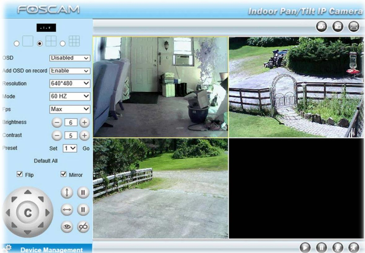
The round dial labeled “C” is your camera rotation control, as are the smaller up-down and side-to-side buttons to the right of it.
